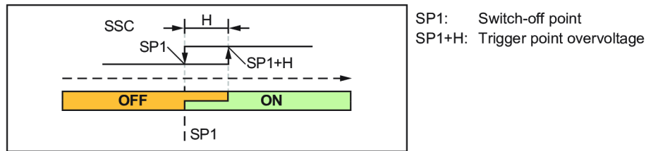
Figure 6: Make contact (IO-Link parameter LoGc: high active)
