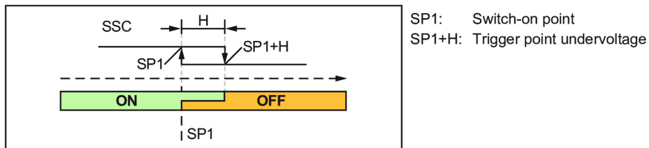
Figure 7: Break contact (IO-Link parameter LoGc: low active)
