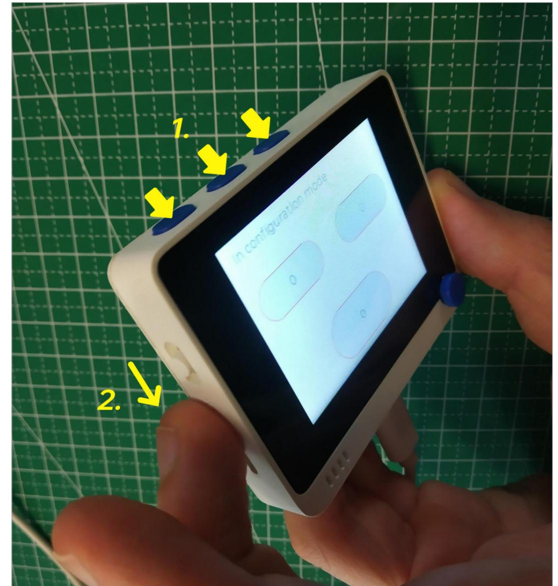
"In configuration mode" will be displayed on device screen. Connect to device with Serial monitor (baud rate 115200, carriage return) and set WiFi SSID, password and Azure IoT Central credentials (in the following format `set_az_iotcyour_ID_scopeyour_primary_keyyour_device_ID`), which you can get by following these steps:
