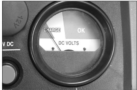
**NOTE:** Pressing the 'TEST' button with the charger disconnected will cause the needle on the battery condition gauge shown above, to register the state of charge of the battery.
