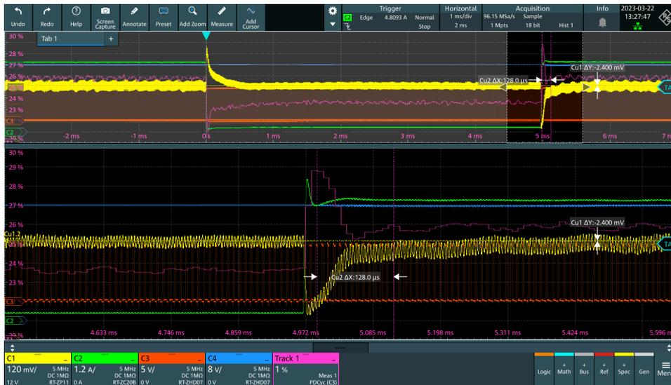
Reviewing control theory shows the 2% deviation comes from higher conduction losses caused by higher output current. The higher losses are mainly generated in the transformer and output rectifier. The additional losses need to be equalized by increasing the positive duty cycle and the track function allows this complex measurement task to be performed.
