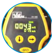
Trips GFCI at 6mA or 30mA
