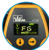
Detects and Displays false or "bootleg" ground
