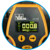
Displays neutral to ground voltage
