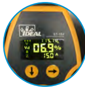
Displays Voltage Drop at 12, 15 & 20 Amps
