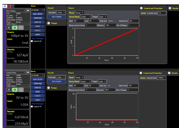
Figure 11- Aim-TTi Test Bridge SMU setup.
