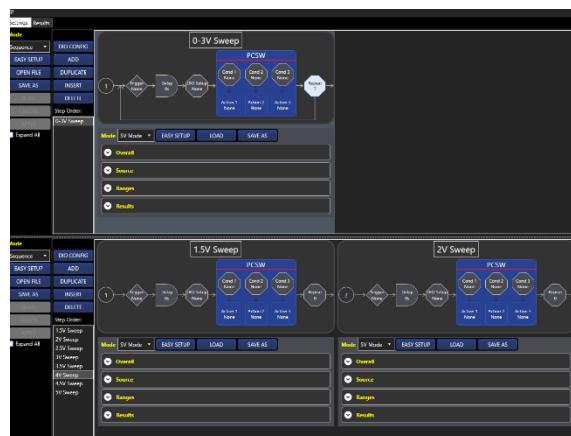
Figure 12- Aim-TTi Test Bridge SMU sequence setup.
