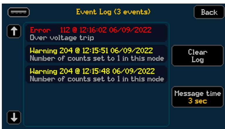
Selecting the Event Log symbol on the status bar will open the event log menu, this menu can also be accessed through the System menu: CNFG > [System] Event Log. Within the Event log menu, the events are colour coded and include a Warning or Error number alongside the time and date of when the error occurred.
