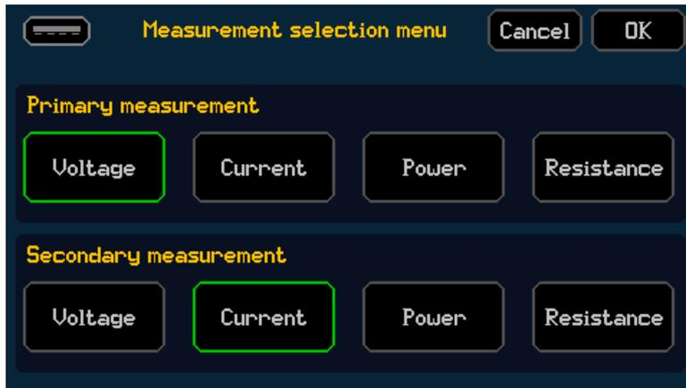
The measurement selection configures the primary and secondary measurements. The primary and secondary measurements can be set to measured voltage, measured current or the computed power or resistance.
