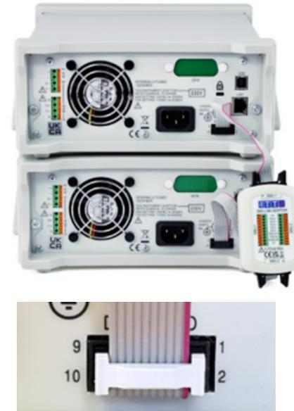
The Link Adaptor mates with standard 10W (2 x 5 DIL) female 2.54mm pitch IDC ribbon cable.
