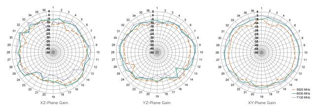
Figure 16. Radiation Patterns for the W63WS1 Antenna on Edge of Ground Plane, Bent 90 Degrees
