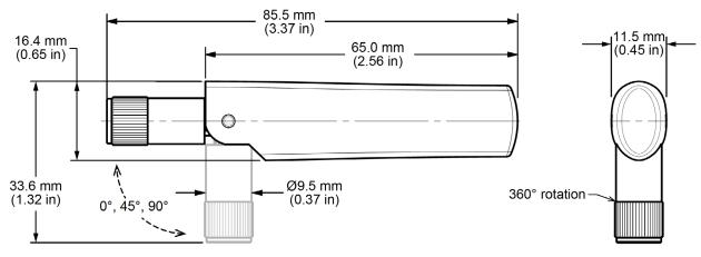
Figure 1. ANT-W63WS1 Antenna Product Dimensions
