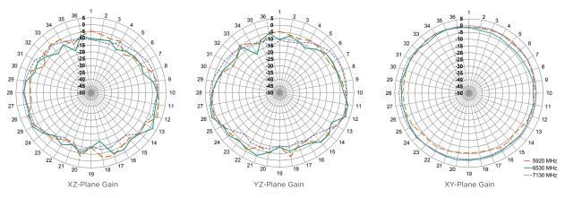
Figure 9. ANT-W63WS1 Antenna Radiation Patterns, Straight
