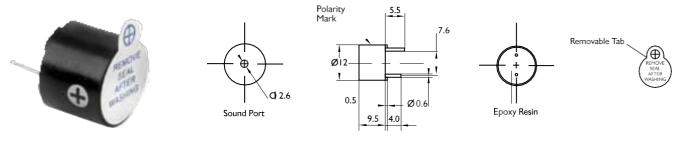
Dimensions : Millimetres Tolerance: ±0.5mm
