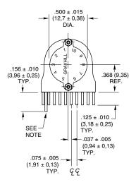
Note: Common location for a single pole per deck switch. For common location on two pole switches see circuit diagrams.
