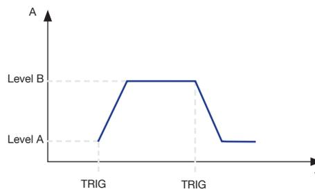
The DC load current will toggle between Level-A and Level-B following receipt of a trigger signal.
