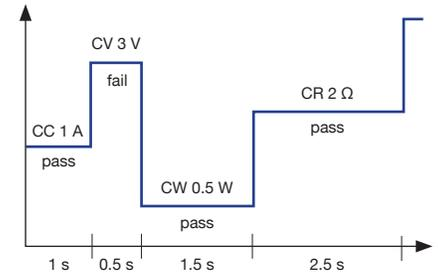
Up to 100 different sequences can be linked to run steps of various operating modes and loading conditions. Each step can be programmed with upper and lower pass/fail limits.
