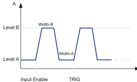
Upon receipt of a trigger signal, the load executes one pulse cycle then returns to load current level A.
