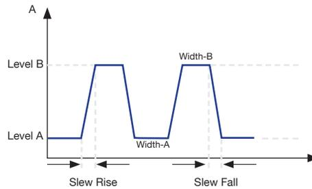
Switch continuously between A and B load current levels where rise/fall slew rates and level width can be adjusted.
