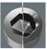
Hexagon socket screws are a problem, because the contact surfaces that transfer the force of the tool to the screw are very narrow. The consequence: the head of the screw can be damaged, usually rounding out the recess. Hex-Plus tools have larger contact surfaces to prevent this, driving from the flats of the recess, rather than the corners. Good to know: Hex-Plus tools fit into every standard hexagon socket screw!
