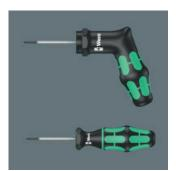
Wera torque-indicators have been factory pre-set to values recommended by leading carbide manufacturers. These tool tightening values relate specifically to the size of the TORX®, TORX PLUS® or hexagon socket screw. Torque indicators ensure safe and loosening easy of screw connections. Precision :  $\pm \ 10 \ \%$
