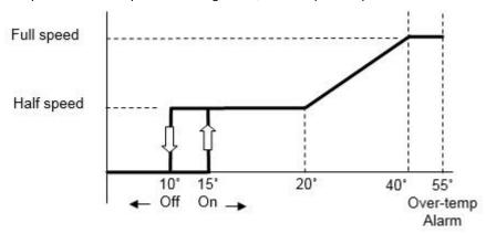
Each fan may have a different profile using either thermistor as configured.
