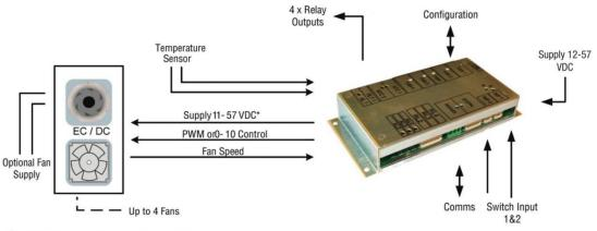
\*For 0-10 V fans, minimal supply voltage is 16 VDC For open collector fans, minimum supply is 11 VDC
