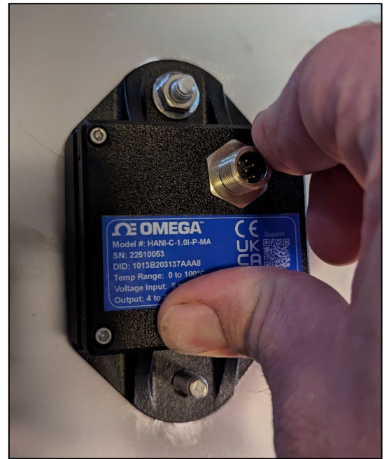
Figure 13: Secure the hardware nuts to properly mount the HANI™ Tank Sensor
