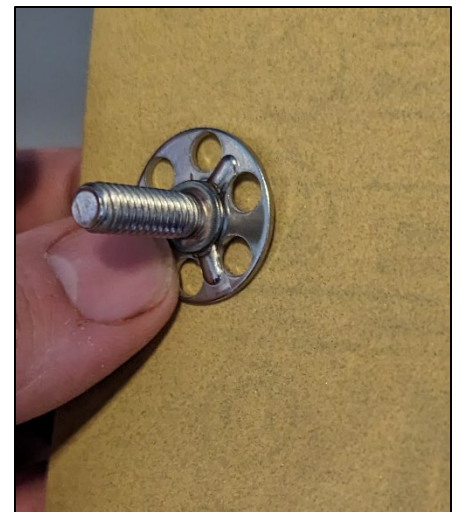
Figure 7: Sand the adhesive studs
