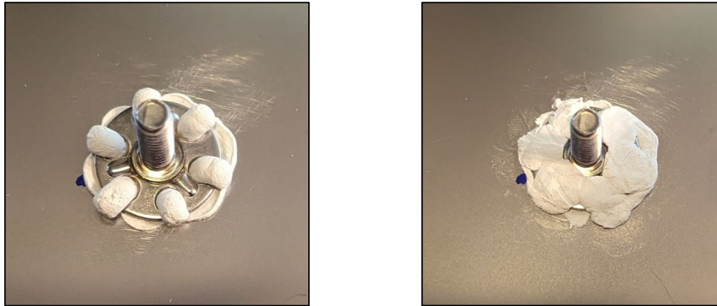
Figure 11: Evenly distribute the epoxy across the top of the stud base
