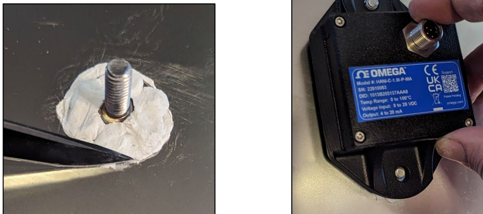
Figure 12: Clean off excess epoxy, test fit, and let cure
