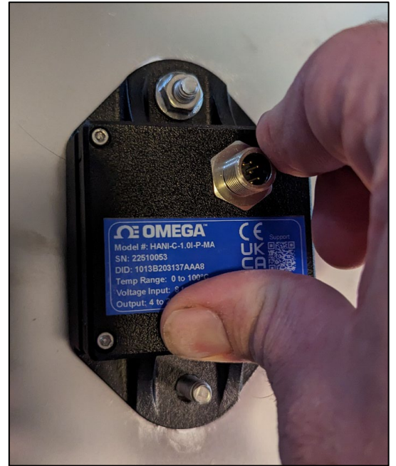
Figure 4: Secure the hardware nuts to properly mount the HANI™ Tank Sensor
