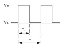
$\begin{array}{l} V_{IH} = 4.75 \ \text{to} \ 5.25 \ \text{V} \quad V_{IL} = 0 \ \text{to} \ 0.4 \ \text{V} \\ \\ \text{PWM duty cycle (\%)} = \frac{T_1}{T} \times 100 \qquad \text{PWM frequency } 25 \ (\text{kHz}) = \frac{1}{T} \\ \\ \text{Current source (Isource)} = 1.0 \ \text{mA max. (when control voltage is } 0 \ \text{V}) \\ \\ \text{Current sink (Isink)} = 10 \ \text{mA max. (when control voltage is } 5.25 \ \text{V}) \\ \\ \text{When the PWM control terminal is open,} \end{array}$
