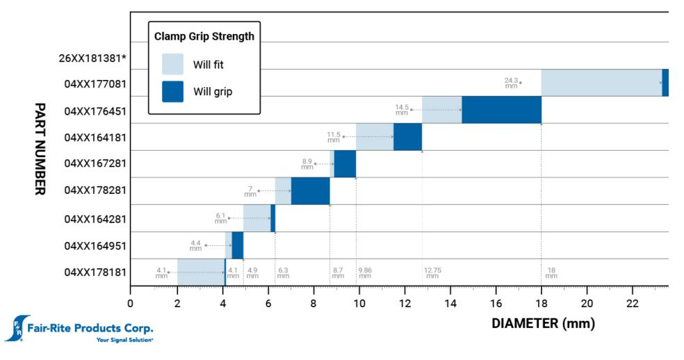
The B dimension is the core inside diameter.
