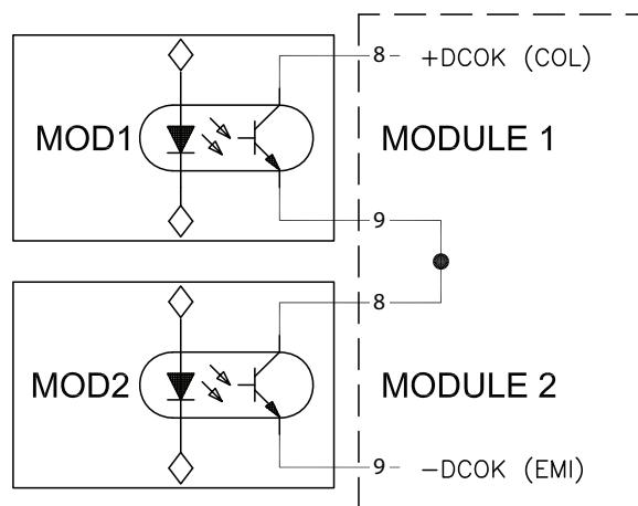
**Use of Module Inhibit for Modules in Parallel or Series**
