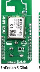
With ultra-low power TCM515 transceiver gateway module and operates at 868MHz radio band.
