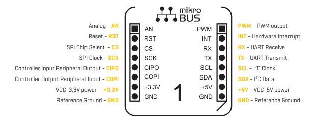
mikroBUS $^{\text{m}}$  - the add-on board socket standard that offers maximum expandability with the smallest number of pins. All the major vendors have accepted the mikroBUS $^{\text{m}}$  standard and added it to their development boards.
