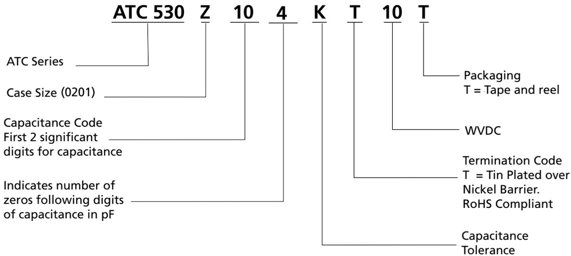
The above part number refers to a 530 Series (case size Z) 100 nF capacitor, K tolerance (±10%), with T termination (tin plated over nickel barrier, RoHS compliant), 10 WVDC, tape and reel packaging.
