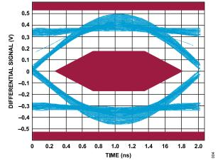
Figure 4. High-Speed, Near-End Device Eye Diagram
