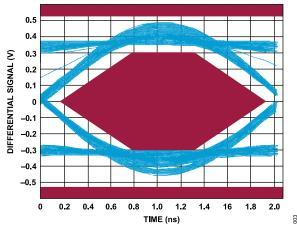
Figure 3. High-Speed, Far-End Device Eye Diagram
