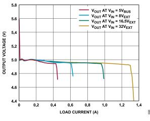
Figure 6. Output Load Regulation Plot
