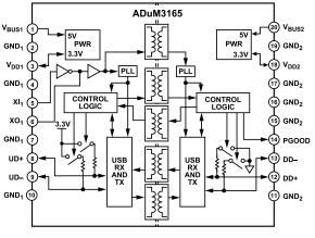
Figure 2. ADuM3165 Functional Block Diagram
