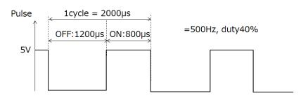
Notes: \*On time (Pulse width): When pulsing the LED, the output becomes stable within 400 micro sec., max. Therefore 800 (>> 400) micro sec. of on time is recommended, to ensure proper operation.
