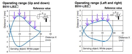
In the case of detecting moving objects, a reflective type sensor is generally mounted vertically to the surface on which the light emitting axis and the light receiving axis are crossing (equal to "Left and right" direction).
