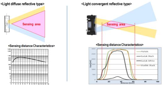
The B5W-LB series is composed of light convergent reflective type sensors utilizing Omron's original optical lenses which are combined with 4-toroidal lens designs. These sensors can provide stable sensing with a small amount of reflected light, and even black paper and transparent plates can be detected in its wide sensing range. Furthermore, the B5W-LB series will not detect any highly reflective background that is positioned beyond the sensor's sensing area.
