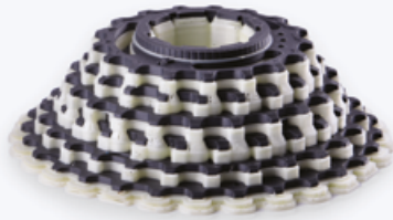
Bicycle cassette model before support material dissolution
