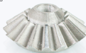
Bevel gear 3D printed with BASF Ultrafuse® 316L after the debinding and sintering procedures
