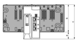
a: additional space below the rack to accommodate the height of the CPU. For an X Bus rack, the value is 30.9 mm (1.217 in.); for an Ethernet rack, the value is 29.49 mm (1.161 in.).
