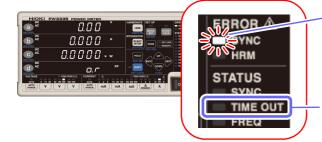
Accurate measurement cannot be performed if the **SYNC** lamp (ERROR) is lit up.
