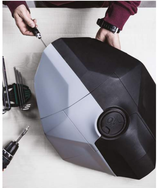
A full scale prototype of a motorbike fuel tank 3D printed on Zortrax M300 Plus with Z-HIPS.
