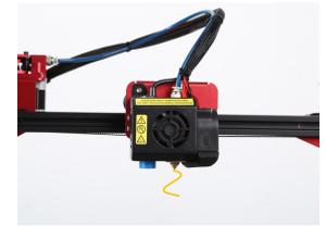
Press and hold the extruder lever and insert the 1.75mm filament through the filament detector and through the extruder motor. Continue feeding until you see filament extrude from the nozzle.
