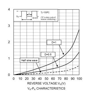
REVERSE POWER DISSIPATION:P<sub>R</sub>(W)
