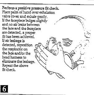
Do not use with beards or other facial hair that prevent direct contact between the face and the edge of the respirator. If you cannot achieve a proper fit, do not enter the contaminated area. See your supervisor or call 3M on 0800 525385 (charge-free line).
