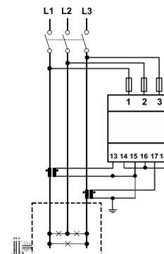
**Fig. 7** Three-phase without neutral (3-wire). MID
