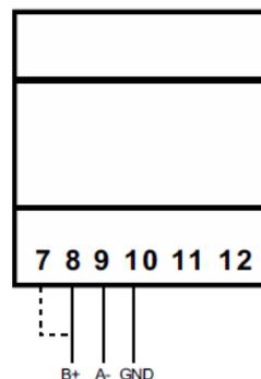
*Fig. 12 Last device on RS485*
