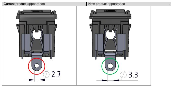
Changed size of terminal holes from 2.7 to 3.3 mm •
