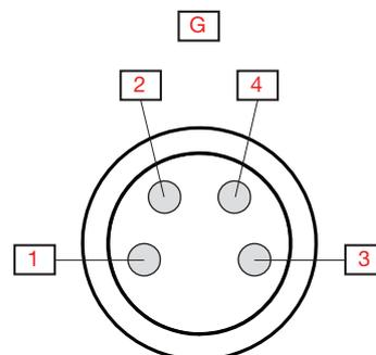
Fig. 3 "M8-plug" Pin numbers
