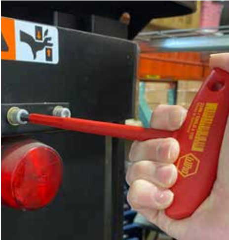
Wiha Insulated T-handle Blade CVM tool steel, hardened to average 58/60RC
