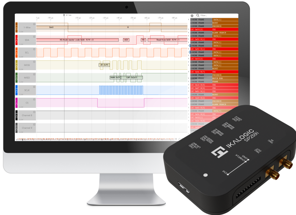
Figure 3: Example of logic signals captured and analyzed by SP259 logic analyzer
