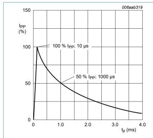
Fig. 1. 10/1000 μs pulse waveform according to IEC 61643-321
