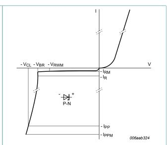
Fig. 2. V-I characteristics for a unidirectional TVS protection diode
