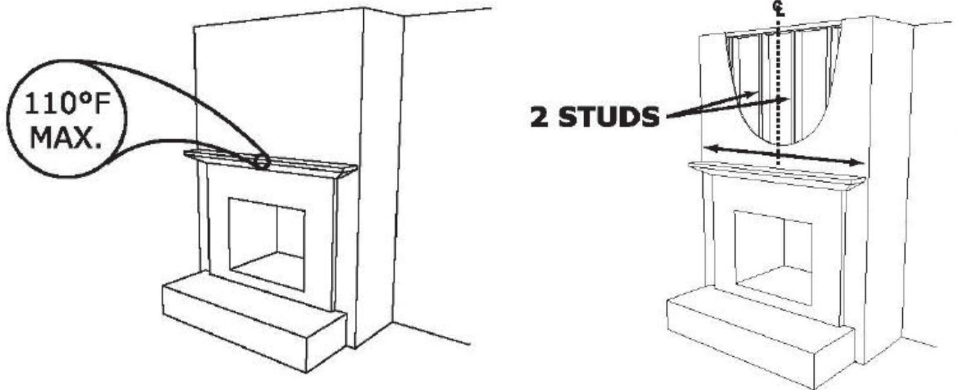
2. The wall to which this mount will be attached must be a wood stud type, with studs spaced no more than 24"(609mm) apart. These studs should be symmetrically positioned or the installation will not be symmetrical to the fireplace mantle. The wall must be no more than 5/8" (16mm) thick.
