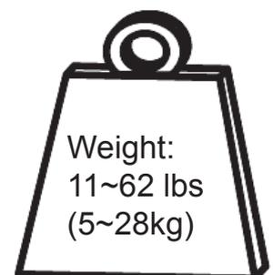
4. This mount is intended for flat screen televisions (LCD, LED, Plasma) only. The mounted television should be between 42 ~ 65" and weigh between 11~62 lbs.
