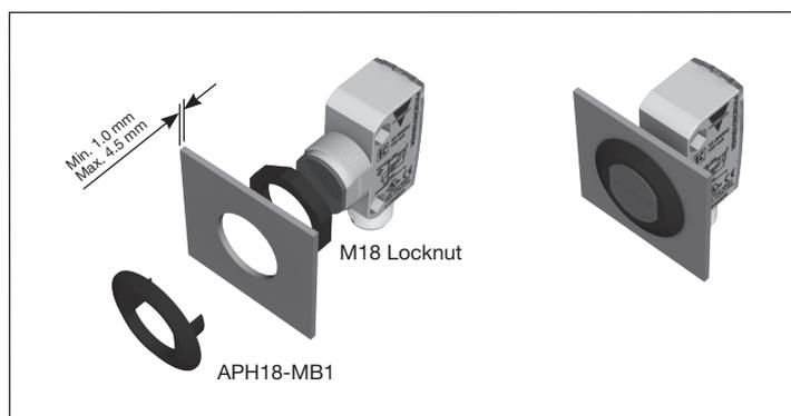
PH18 mounting with a combination of 1 x APH18-MB1 and 1 x M18 locknut.
