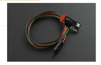
digital high/low level(low when liquid detected) and adopts 3-pin DuPont connector, which can be widely used in water tank detection, beverage machine, water pipe level detection, scientific experiment test tube level detection and other scenarios.
