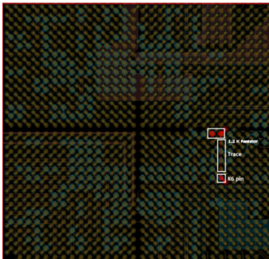
Figure 2-6. Component Between 1.2 K Resistor and K6 Pin
