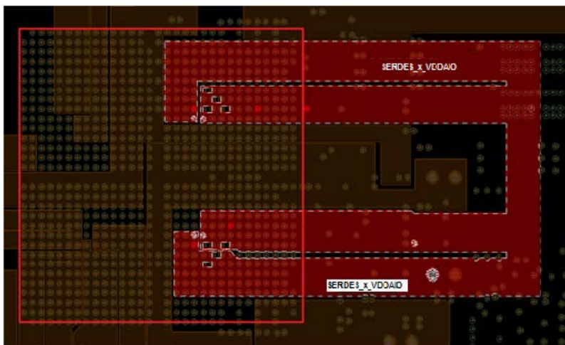
Figure 2-8. Layout of SERDES_x_VDDAIO Plane
