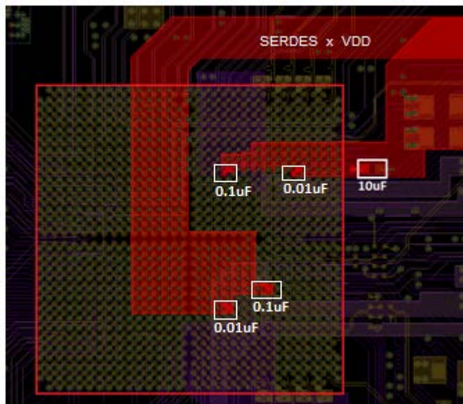
Figure 2-7. Layout for SERDES_x_VDD Plane
