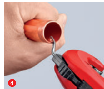
4 and you're done! If necessary, have the edge smoothed out using the fold-out deburring tool – with surprisingly little effort
