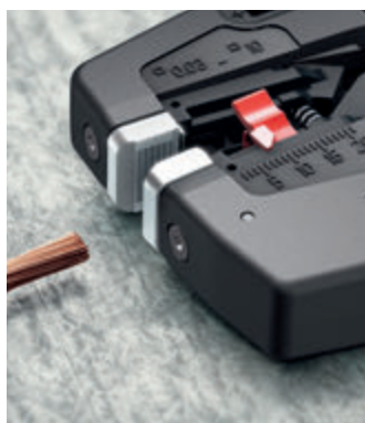
Automatic stripping up to 10 mm 2 .
