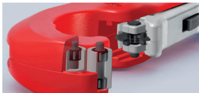
High-quality needle bearings enable the cutting wheel and the four guide rollers to operate virtually without any friction during the cutting – cuts stainless steel pipes with particular ease
