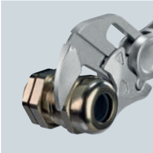
Large capacity, precise grip: As the jaws always grip in parallel, the Pliers Wrench XS is particularly gentle on hex heads with decorative finishes in sizes up to 21 mm width across flats.
