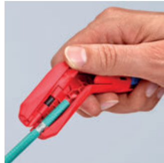
Stripping of a data cable
