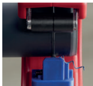
Segments as short as 10 mm can be cut. The spiral chip comes from chamfering
