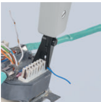
Inserts and cuts cables in one operation
