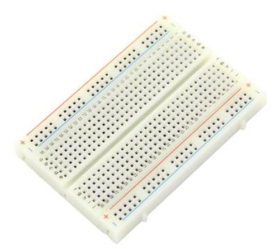
**Breadboard** is a prototyping device for electronic circuits. It is very useful to connect electronic components and to make a circuit without soldering. Breadboard consists of rows and columns of holes with metal contacts to insert components. The breadboard supplied with Arduino Sidekick Basic Kit is arranged of **2 X 30 five-hole** columns and **4 X twenty five-hole** rows. These holes are connected internally in a manner as illustrated below.
