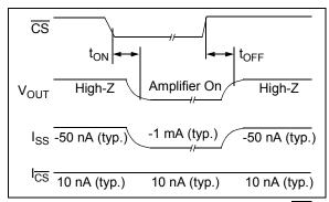
**FIGURE 1-1:** Timing diagram for the  $\overline{\text{CS}}$  pin on the MCP6023.
