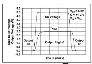
**FIGURE 2-39:** Chip Select  $(\overline{CS})$  to Amplifier Output Response Time (MCP6023 only).
