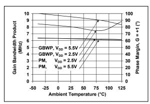
**FIGURE 2-21:** Gain Bandwidth Product, Phase Margin vs. Temperature.
