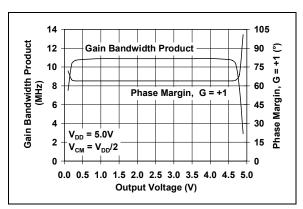
FIGURE 2-24: Gain Bandwidth Product, Phase Margin vs. Output Voltage.
