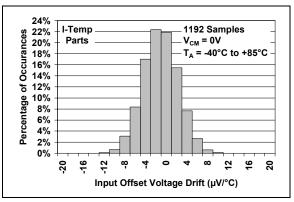
**FIGURE 2-4:** Input Offset Voltage Drift, (Industrial Temperature Parts).
