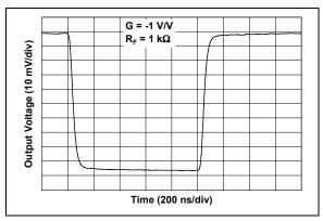
FIGURE 2-35: Small-Signal Inverting Pulse Response.
