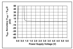
**FIGURE 2-37:** V<sub>REF</sub> Accuracy vs. Supply Voltage (MCP6021 and MCP6023 only).
