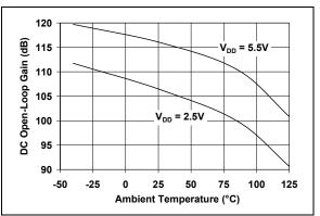
**FIGURE 2-22:** DC Open-Loop Gain vs. Temperature.
