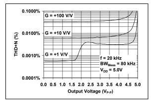
**FIGURE 2-29:** Total Harmonic Distortion plus Noise vs. Output Voltage with f = 20 kHz.
