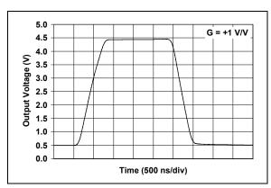
**FIGURE 2-33:** Large-Signal Non-inverting Pulse Response.
