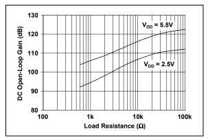
**FIGURE 2-19:** DC Open-Loop Gain vs. Load Resistance.
