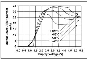
**FIGURE 2-15:** Output Short-Circuit Current vs. Supply Voltage.
