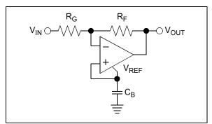
**FIGURE 4-8:** Inverting gain circuit using V<sub>RFF</sub> (MCP6021 and MCP6023 only).
