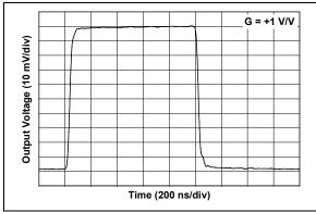
**FIGURE 2-32:** Small-Signal Non-inverting Pulse Response.
