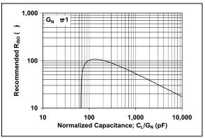
**FIGURE 4-3:** Recommended  $R_{ISO}$  values for capacitive loads.
