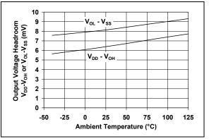
**FIGURE 2-34:** Output Voltage Headroom vs. Temperature.
