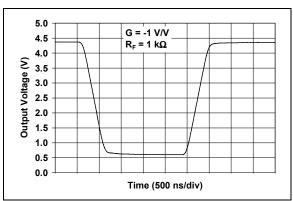
FIGURE 2-36: Large-Signal Inverting Pulse Response.
