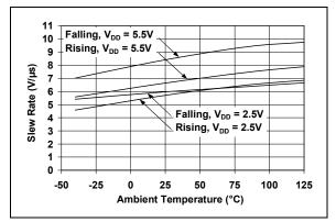
FIGURE 2-25: Slew Rate vs. Temperature.
