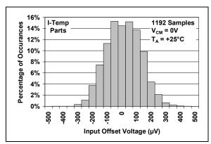
FIGURE 2-1: Input Offset Voltage, (Industrial Temperature Parts).
