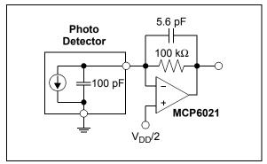
**FIGURE 4-12:** Transimpedance Amplifier for an Optical Detector.
