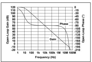
**FIGURE 2-18:** Open-Loop Gain, Phase vs. Frequency.
