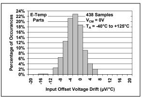
**FIGURE 2-5:** Input Offset Voltage Drift, (Extended Temperature Parts).
