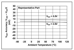
**FIGURE 2-40:** V<sub>REF</sub> Accuracy vs. Temperature (MCP6021 and MCP6023 only).
