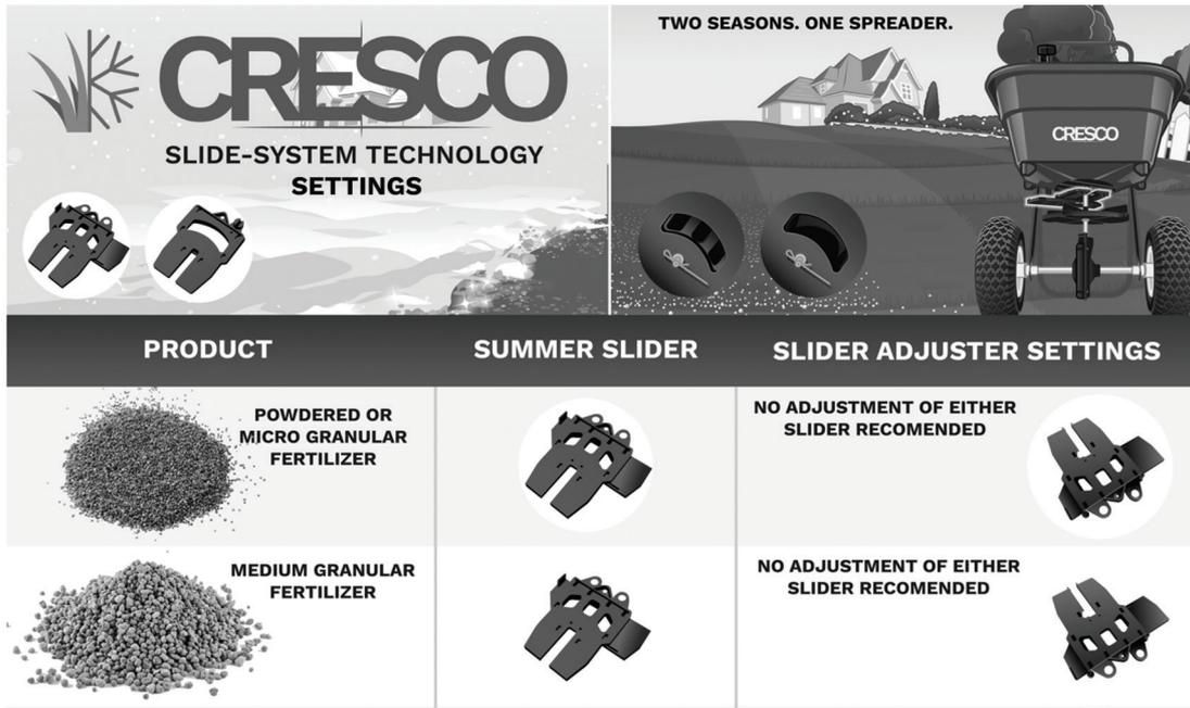
The chart is titled "CRESCO SLIDE-SYSTEM TECHNOLOGY SETTINGS" and "TWO SEASONS. ONE SPREADER." It provides settings for two types of fertilizers: powdered or micro granular, and medium granular. For both, it states that no adjustment of either slider is recommended. The chart includes images of the fertilizer types and the corresponding slider settings.
