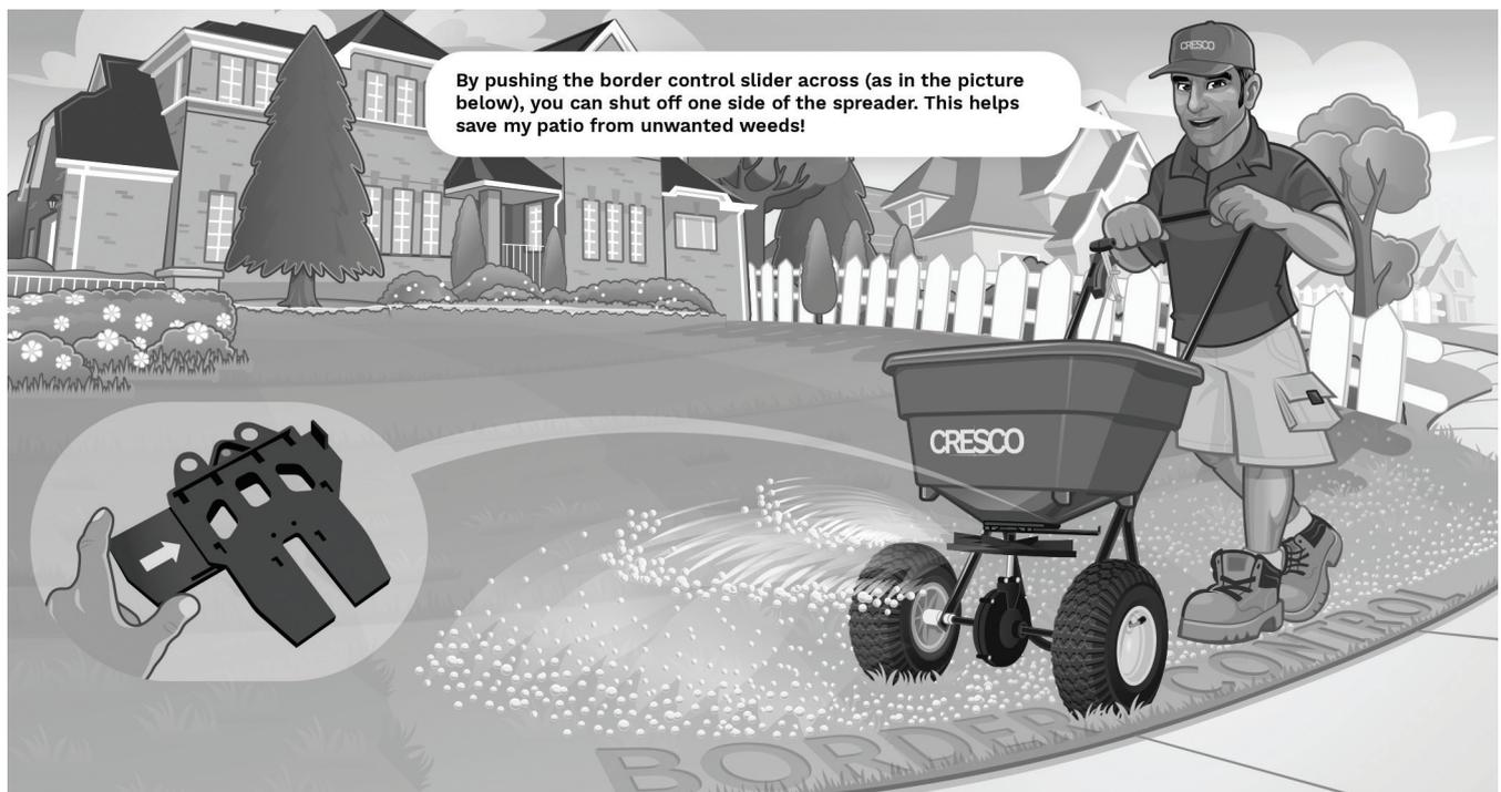
To protect your borders simply slide the border control into position to cut off the left hand side of the spread pattern.
