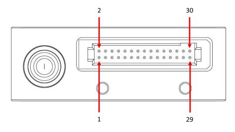
The following table describes all the interface pins. Contact Broadcom for additional information on the auxiliary interface.
