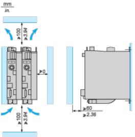
LXM32•U45M2, •U90M2 and LXM32•U60N4 servo drives are cooled by natural convection. LXM32•D18M2, •D30M2, LXM32 •D12N4, •D18N4, •D30N4 and •D72N4servo drives have an integrated fan. When installing the servo drive in the enclosure, follow the instructions below with regard to the temperature and protection index:
