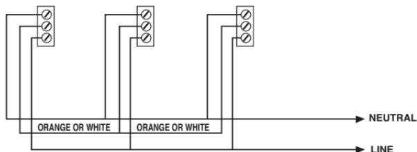
**FOR INTERCONNECT: USE STANDARD 3 core & earth cable 1.5mm<sup>2</sup> cable**
