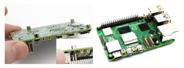
3. Insert the board into the case and tighten the 4 screws from the bottom side.
