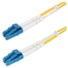
OS2 LC to LC Single Mode Duplex Fiber Optic Patch cable facilitates connectivity across 10G networks. It supports Coarse Wavelength Division Multiplexing (CWDM) across an extended wavelength range of 1260-1625nm, improving channel isolation for optimal signal strength over long distances.
