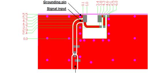
Transmission Line with 50Ω Impedance Characteristic
