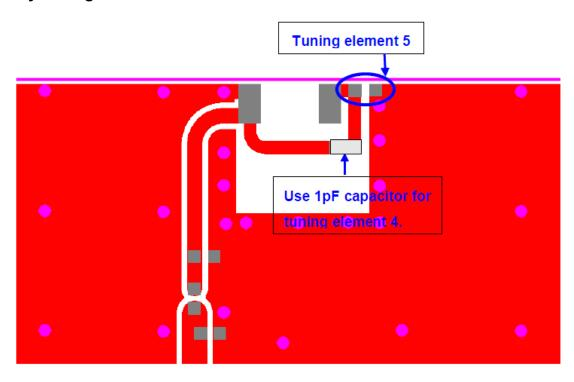
1575.42 MHz GNSS Chip Antenna
